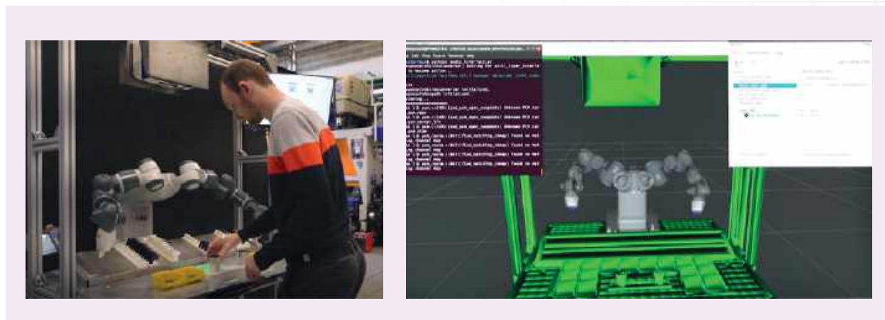
Figure 5. (Left ) An assembly station with an operator, (right) a real-time digital twin derived from and updated with world model data.
